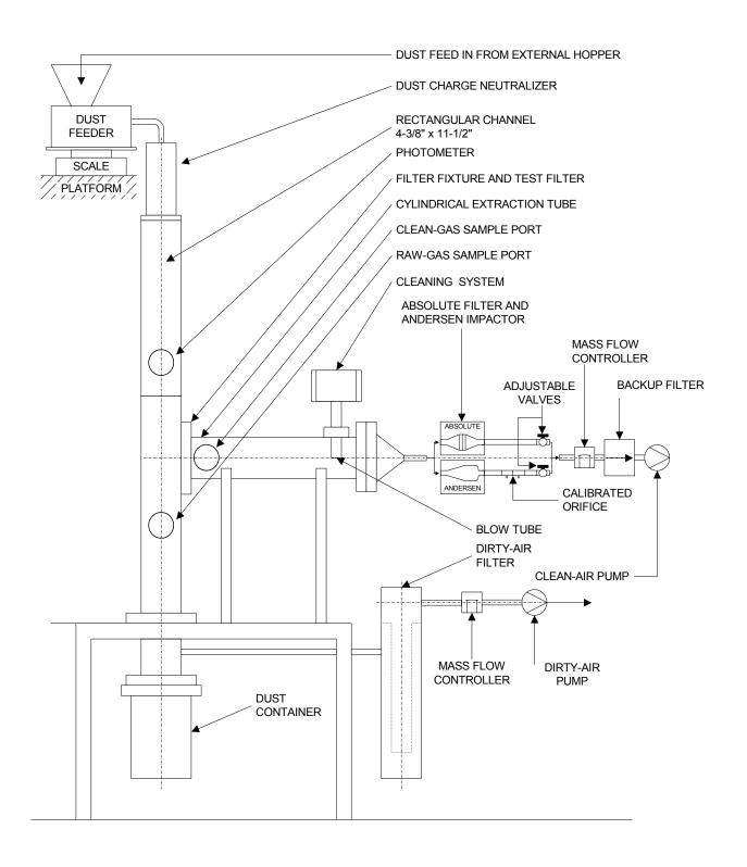
Figure 1 Filtration Performance Test Apparatus
